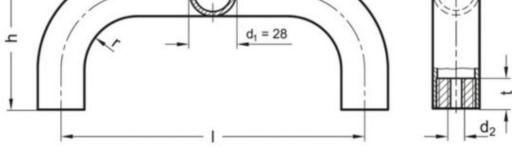
$\begin{array}{ll} d1 &= 28 \\ d2 &= M10 \\ h &= 78 \\ I &= 350 \\ r &= 32 \\ t \mbox{ min} = 15 \end{array}$
